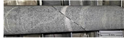
Fig 3. Fracture displacement at 936.84 m depth (KBH-3)
